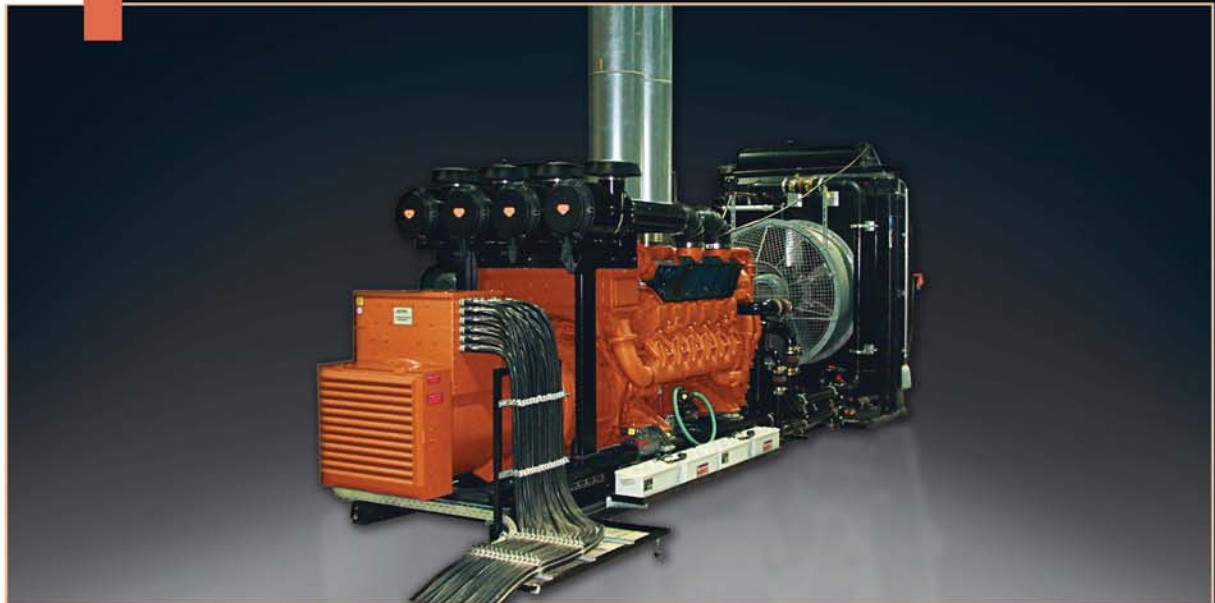
D 1400-4 MWE standby system, output of 1400 kVA, for supplying emergency power to a clinic.
